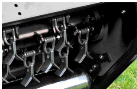
Y-shaped mounting of knives on shackles
