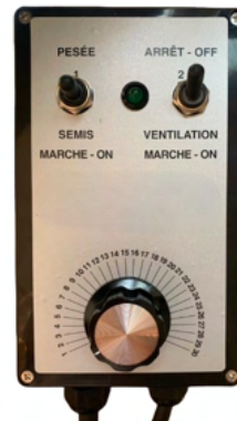
Seed flow adjustment via the graduated dial
