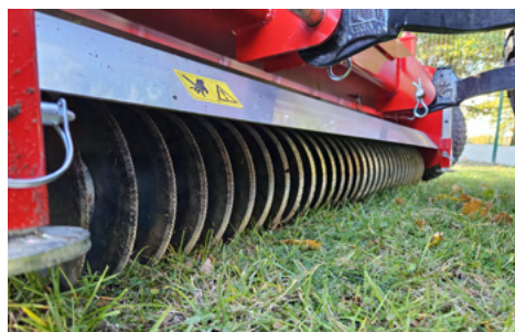
Sharp discs for stress action on weeds
