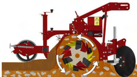
Soil preparation principle
