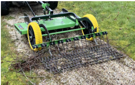
Rake, harrow and grid for clod crumbling
